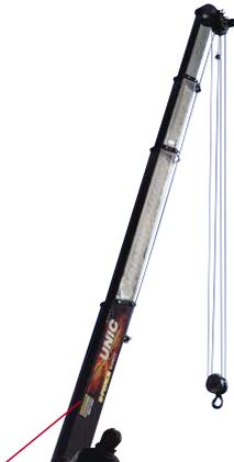
傾斜角度計視認用LED作業灯
